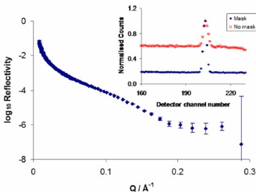
Reflectivity curve for a sapphire/D<sub>2</sub>O surfactant solution interface. The inset shows the comparison of total counts for similar measurements with an absorbing blade to reduce background (blue) and without blade (red).
