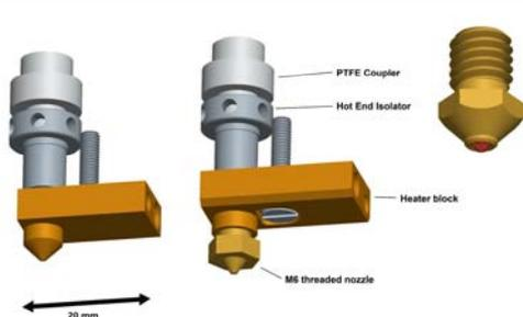
New printer nozzles with ruby inserts have been developed, designed to cope with hard materials such as boron carbide composites [2]. The nozzles are now available commercially.
