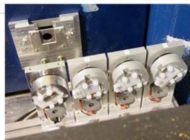
Apertures for small-angle scattering that give low background by using <sup>10</sup>B<sub>4</sub>C composite. The observed scattering for the <sup>10</sup>B<sub>4</sub>C composite is approximately the same as that for a cadmium aperture [1], shown below.
