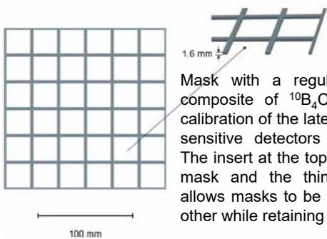
Mask with a regular array of absorbing composite of <sup>10</sup>B<sub>4</sub>C in ABS designed for calibration of the lateral response of position-sensitive detectors for neutron scattering. The insert at the top shows the profile of the mask and the thinner edge section that allows masks to be placed adjacent to each other while retaining a uniform array.
