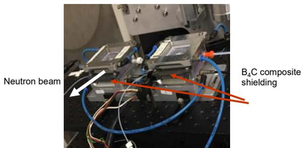
Reflection cells on Inter Reflectometer sample stage at ISIS. <sup>10</sup>B<sub>4</sub>C composite neutron absorber blades reduce background, data shown below.
